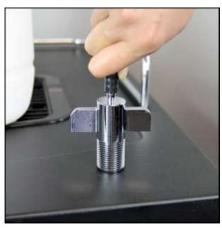
Insert the hose nipple of the Duplex Coupler (3) into the other end of the Plastic Tube. Press down on a hard surface until the tube touches the flat part of the Duplex Coupler.
